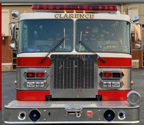
Make: Simon-Duplex (Cab) – Marion (Box) Type: Heavy-Duty Walk-In Rescue with Command Station Engine: Cummings LT A10 Transmission: Allison HT 740 Generator: Winco PTO-Driven GVWR: 42,000 lbs. Wheelbase: 11'-6" Miles: 53,525 Engine Hours: 2,464
